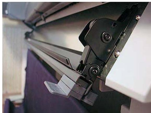
*Manual paper cutter in raised position (left) and in lowered position (right)*
