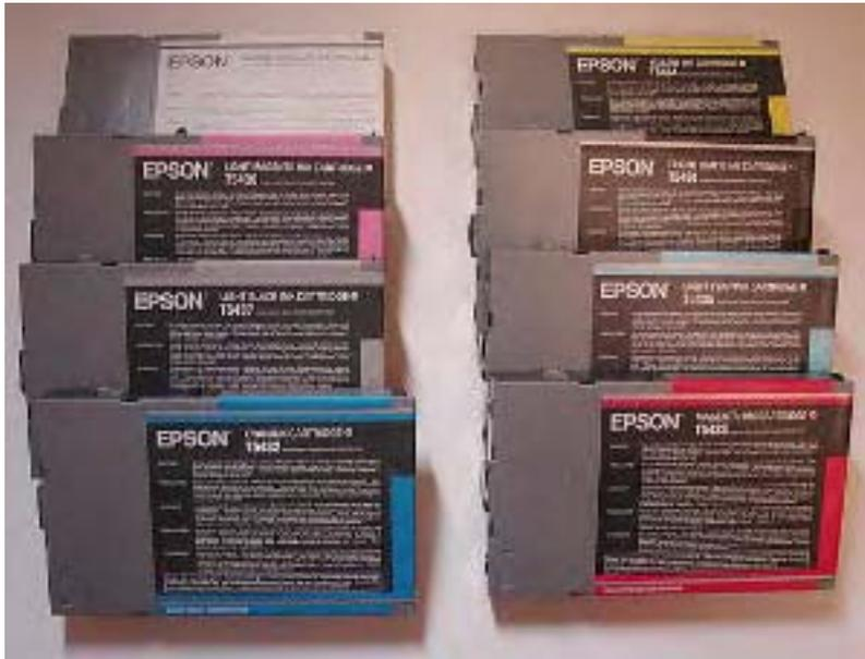
performed the same viewing test with images printed on the Epson 10,000 and could see some amount of green shift on the 10,000 prints, especially in middle grey areas. Epson did improve the firmware for the 10,000 and 7500 in order to reduce metamerism, namely by changing the firing order of the print head, but although this reduced the problem it did not eliminate it completely. The new Ultrachrome inks are, in my estimate, a complete solution to the metamerism problem.
