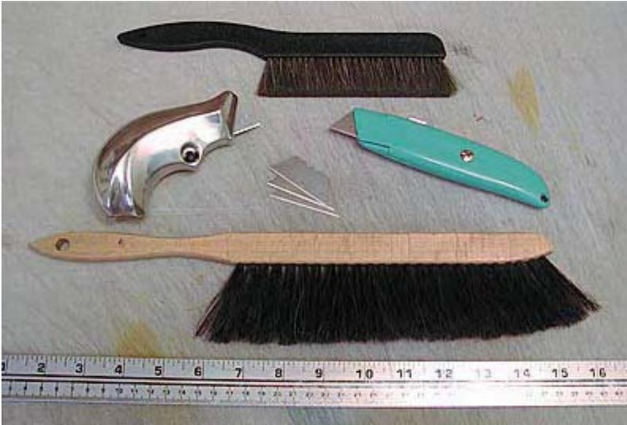
From top to bottom and left to right we have first, an anti-static cleaning brush from Kinetics. This brush will clean the print while removing anti-static electricity. Static tends to attract more dust to the print so this is important. Make sure you clean both the front and the back of the print. When dry mounting the back is actually more important since this is where dust will be trapped in the adhesive and create bumps on the print surface.
