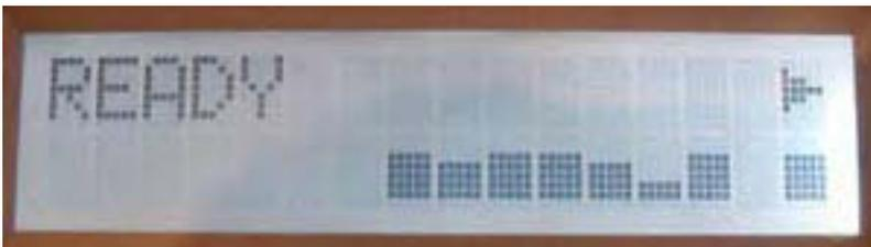
*The the LCD screen on the printer control panel shows a visual display of each cartridge level at all times.*
