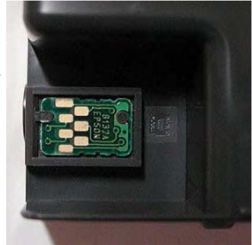
Another item that is chipped is the “maintenance tank”. The purpose of this tank, located on the right side of the printer just above the stand is to collect ink purged from the printhead during either cleaning, cartridge replacement, or cartridge removal (when the printer is to be moved
