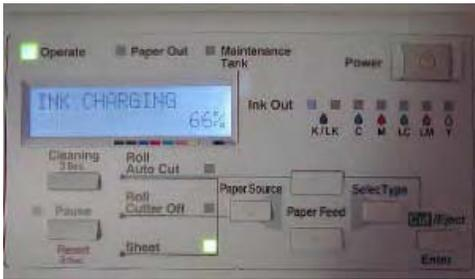
The printer then proceeds to load the ink and keeps you updated of the process on the control panel:
