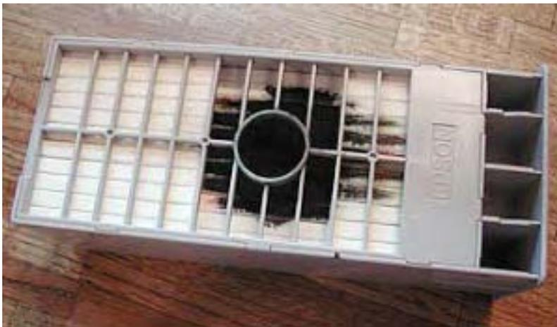
*My maintenance tank. When this photo was taken the tank was “full” according to the printer. Thanks to the hidden “reset” command I am able to continue using this tank.*
